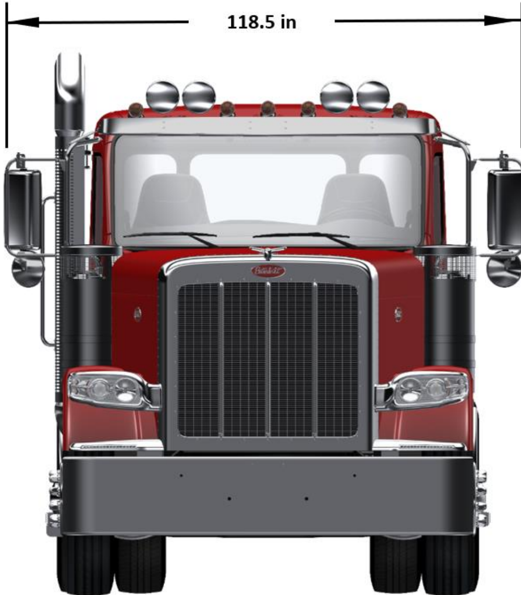
FIGURE 3-3. Model 589-121 Front View – Overall Dimensions
