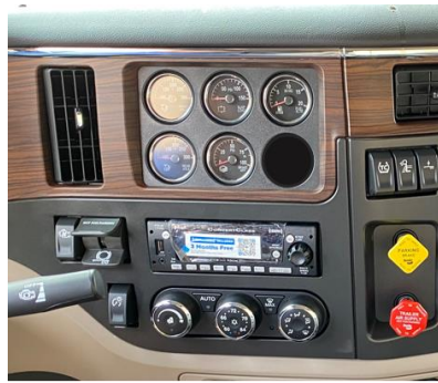
FIGURE 11-4: Dash Panel ready for F/O Fuel Pressure Gauge
